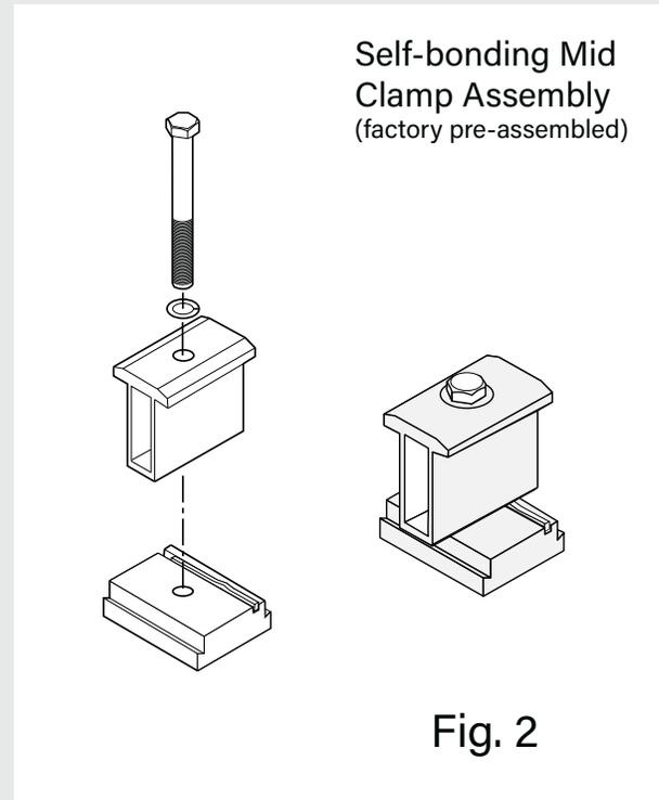
After the support rails have been fastened, you are ready to install the solar modules. There are two sets of clamps: the outside clamps (end clamp) (Fig. 1), and the inter-module clamps (mid clamp) shown (Fig. 2) that install between the modules.
