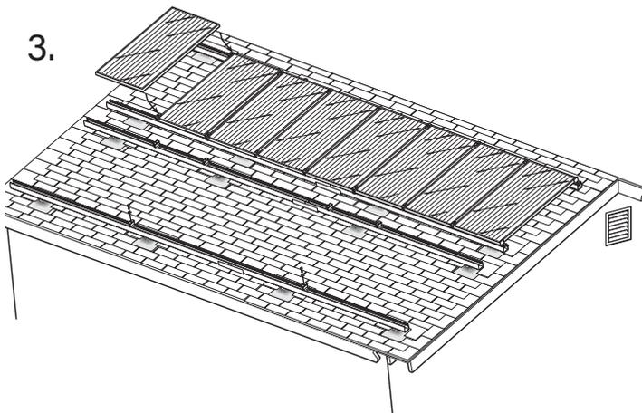
Upon installation of the last module in the panel, install the module end clamp to the end of the last module. We recommend a torque of 15 foot pounds after the last module has been installed and the array has been adjusted/squared. Fully torque mid-clamps before end clamps.
