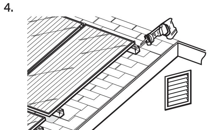
To complete the installation, cut off any excess support rail not being used with a reciprocating saw. Use a file to remove any sharp edges. Per UL2703, it is recommended to periodically re-inspect systems for any loose components or corrosion. Retighten or replace components as necessary.
