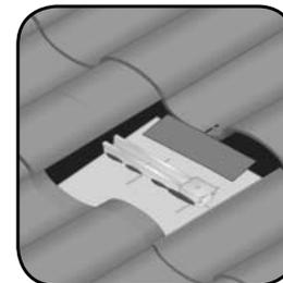
Step 7: Install subflashing and seal as needed if double flash is desired.
