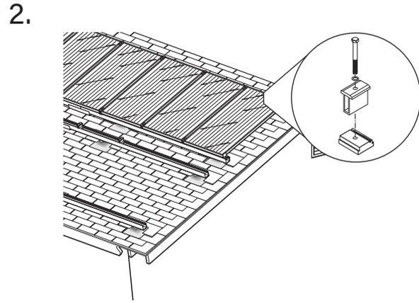
After the first module is secured, slide two mid clamp sets onto the first module side frame. They are designed to stay in place, allowing you to slide and align the next module into place. Repeat this procedure until all modules are installed onto support rail.
