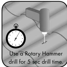
Step 10: Using a 1/2" carbide drill bit and ROTARY HAMMER DRILL in hammer mode, drill through the tile. See online video at [www.prosolar.com](http://www.prosolar.com) for details.
