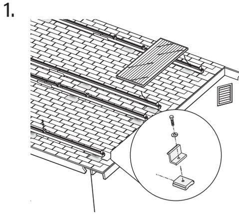
Slide the two end clamps near the end of the support rail and install your end module first. Carefully square the module to the frame and tighten the clamps using a 1/2" deep socket.
